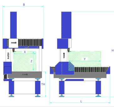
Space requirement sketch relating to mounting of the RAPID-Plus CNC measuring machine.
