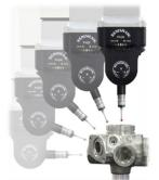
PH20's unique 'head touches' allow measurement points to be taken by moving only the head rather than the CMM structure. Using only the rapid rotary motion of the head, points can be taken faster, and with improved accuracy and repeatability. Furthermore, 5-axis motion eliminates time spent indexing the head. Together these speed increases typically result in a 3fold improvement in throughput over conventional systems.
