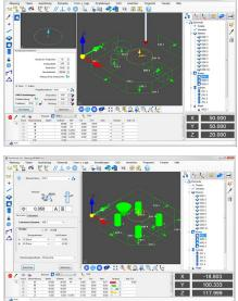
The measurement results are displayed directly in the result window with graphical trend bars.
