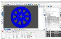
CAD files in IGS and STEP format can be imported. Elements can be selected via the CAD file with one click and automatically measured.
