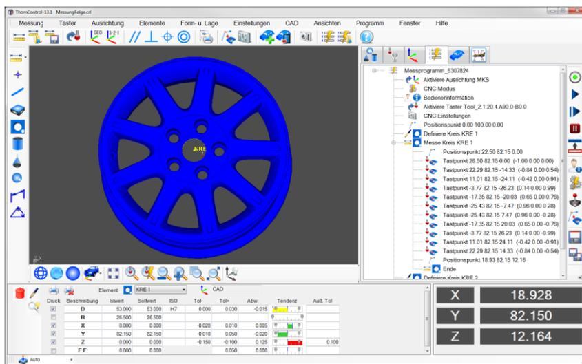
CAD files in IGS and STEP format can be imported. Elements can be selected via the CAD file with a mouse click and automatically measured. The software proposes a measurement strategy and shows the paths graphically. The strategy may be modified as required.
