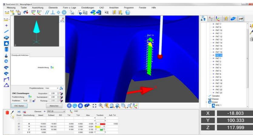
The alignment over 6 surface points and the best-fit alignment are available for fast and accurate alignment against a CAD-part.
