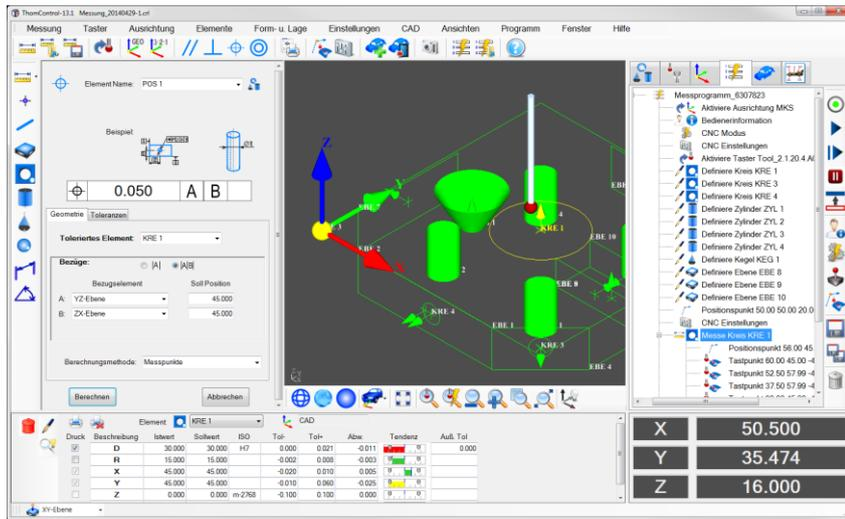
All measurement results are stored and are available again at any time. In addition to the internal file format of THOMControl the measurement reports can also be saved in **Word, Excel and PDF**. The measurement reports are easy to adapt to your layout requirements. Several standard report templates are included.
